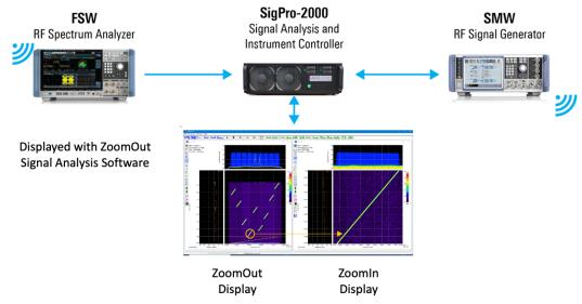
In the above diagram the FSW RF Spectrum Analyzer is providing data to the SigPro-2000B in IQ streams with bandwidths up to 1GHz IBW. The ZoomOut® software suite provides ZoomIn® capability of bandwidths as narrow as 1MHz or less. Captured data can be re-transmitted via the SMW RF Signal Generator at the center frequency selected by the user.
